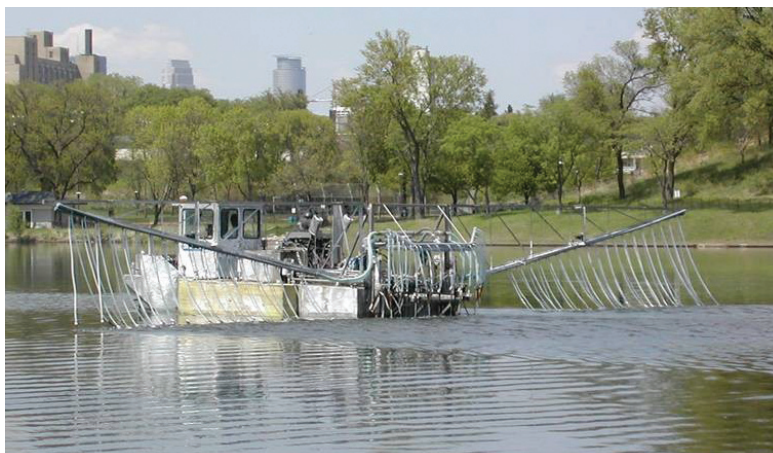
A 2003 Powderhorn Lake alum treatment helps clear phosphorus from the water. Multiple water improvement techniques used by the City and the Minneapolis Park and Recreation Board over the past years are producing results. Powderhorn Lake is now clear enough to support aquatic vegetation.
